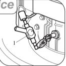
Check the spark plug gap with a feeler gauge and set at 0.76mm.
